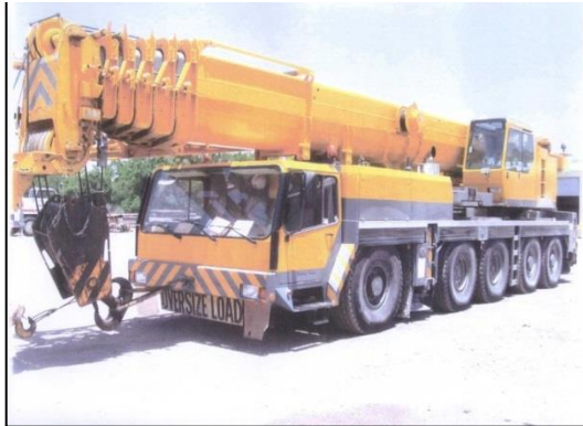
1997 Liebherr LTM1120-165 Ton All Terrain Crane, 184' Main Boom, 37' - 69' Bi-fold Jib w/ 23' Insert for total of 92' Jib, 2 Winches, Liebherr Diesel Engines, 16R25 Tires, 10x6x8, Drive Dolly Prepped .. $575,000.00
