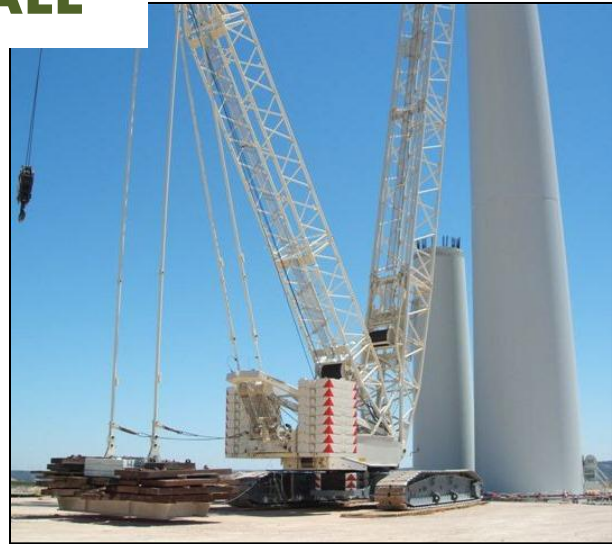
2008 Demag CC2800-1 NT-600T Lattice Boom Crawler Crane, 84M boom, 84M luffing jib, 12M LF2 Fixed Fly Jib, Mercedes, Superlift, 3 drums.... Please Call
