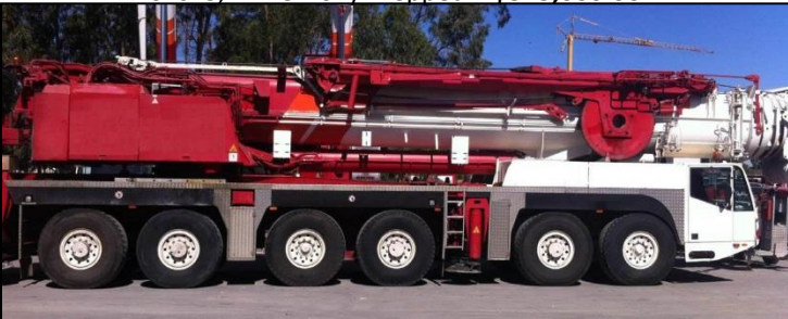
2003 Terex Demag AC350-350T All Terrain Crane w/ SSL Sideways Superlift, 56M boom, 18.1M Jib, 71.6M Luffing, SSL, Daimler Chrysler, 12x8x10, 16.00R25 Tires... Please Call
